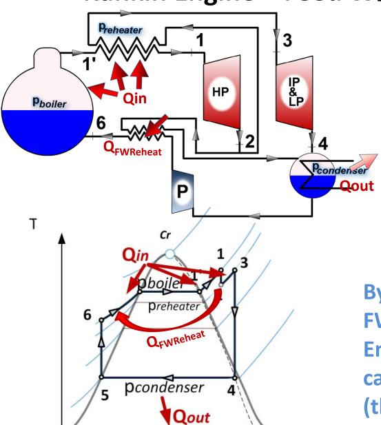
Part of the steam is redirected off from the turbine to heat up the feed water before it enters the boiler.
